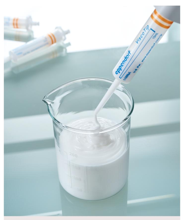
Have you ever experienced the limits of your tips and tools when handling highly viscous liquids? The Repeater® multi-dispenser tip ViscoTip® is specialized for tough-to-handle liquids like cream. Therefore, ViscoTip naturally expands the broad range of applications for our often copied, never equaled Repeater/Combitips® advanced system. For fast, precise and safe liquid handling.
