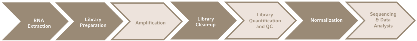
Figure 1: Automated workflow for the Illumina® Stranded mRNA Prep kit on the epMotion® 5075t NGS Solution. Steps highlighted in dark brown can be automated on the epMotion® liquid handler.
