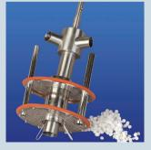
Packed-bed impeller optimizes yields of secreted products; basket is filled with Fibra-Cel® disks and used with a patented low shear draft tube impeller
