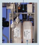
Optional glycol heat exchanger enables rapid cool-down; closedloop, eco-friendly design reduces need for single-pass cooling water through the system
