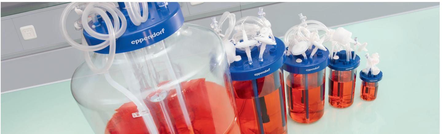
The differently sized bioreactors have similar geometries
